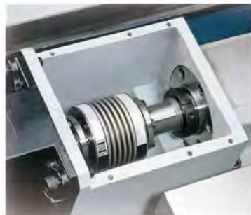
■ Flexible coupling ensures the smooth and accurate movements of the machine
