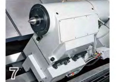
■ High rigidity and strength programmable tailstock
