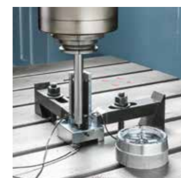
Thermal growth compensation device for spindle
