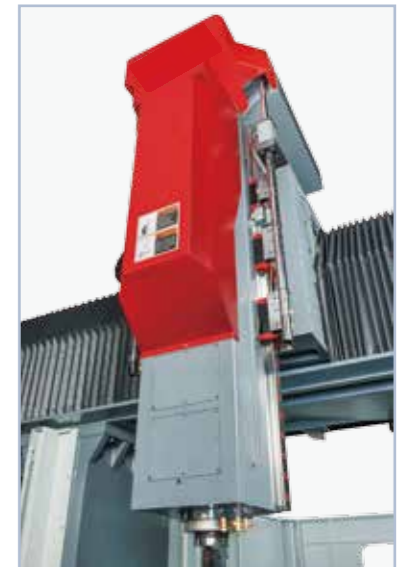
Available to mount with linear guideways on Z-axis and use direct-drive high speed spindle (8,000~15,000 rpm) (optional).
