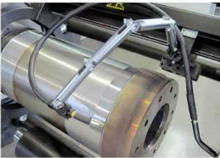
External Overlay welding
