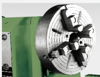
四爪夾頭 4-Jaw independent chuck
