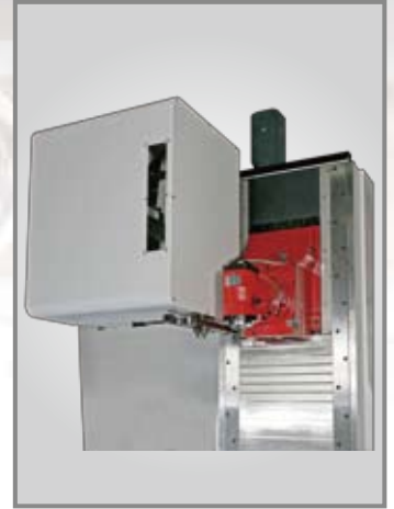
3. 24 stations fixed on traveling column, vertical tool change.
