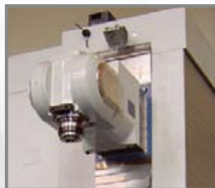
VH-F fork type milling head, HSK-A100 / 34KW / 42KW / 160Nm / 220Nm / 10000RPM / +/-105°
