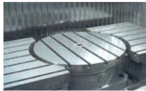
1. \Phi 610\text{mm} / \Phi 800\text{mm} / \Phi 1000\text{mm} rotary table integrated into standard long fixed table.
