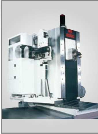
1. 24 station fixed on traveling column, horizontal tool changer
