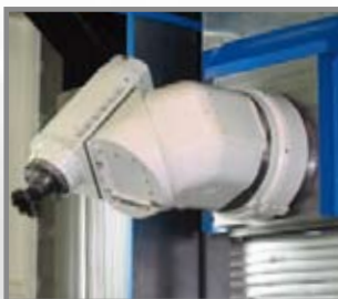
VH-U universal type milling head, HSK-A100 / 34KW / 42KW / 160Nm / 220Nm / 10000RPM
