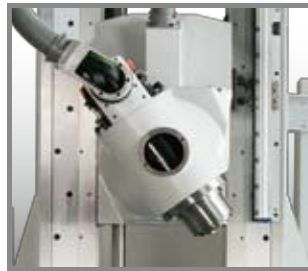
VH-S swivel type milling head, BT#40 / 29.3KW / 35KW / 70Nm / 160Nm / 14000RPM / +/-110°
