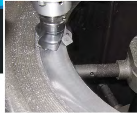
Creation of gasket housing ( MILLING MACHINE with inserts of 60mm)
