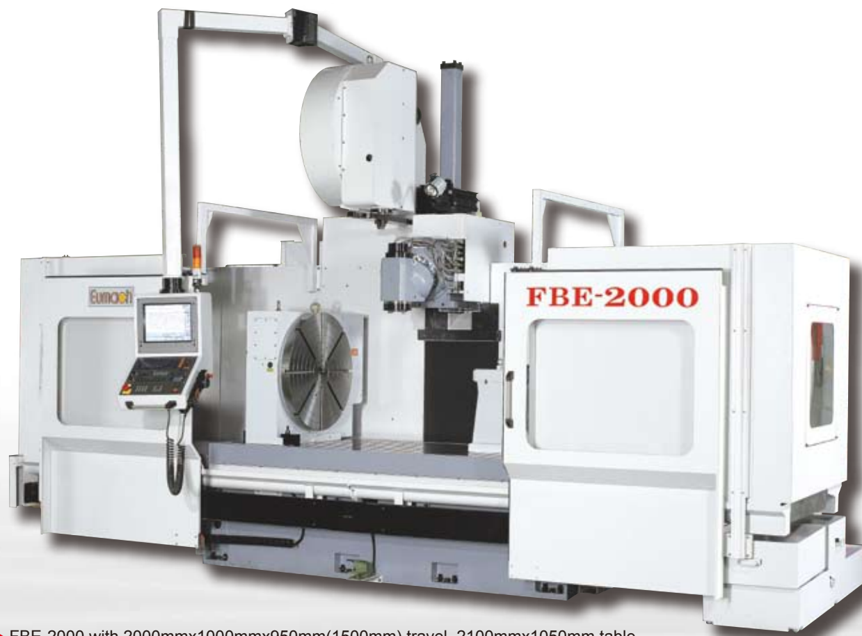
► FBE-2000 with 2000mmx1000mmx950mm(1500mm) travel, 2100mmx1050mm table
