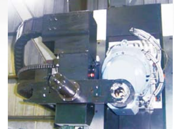
Horizontal tool change with 32, 40 or 60 stations swing arm rail type
