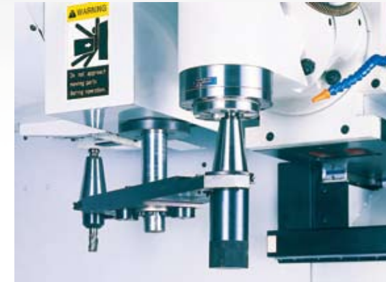
Vertical tool change with 24 stations swing arm type
