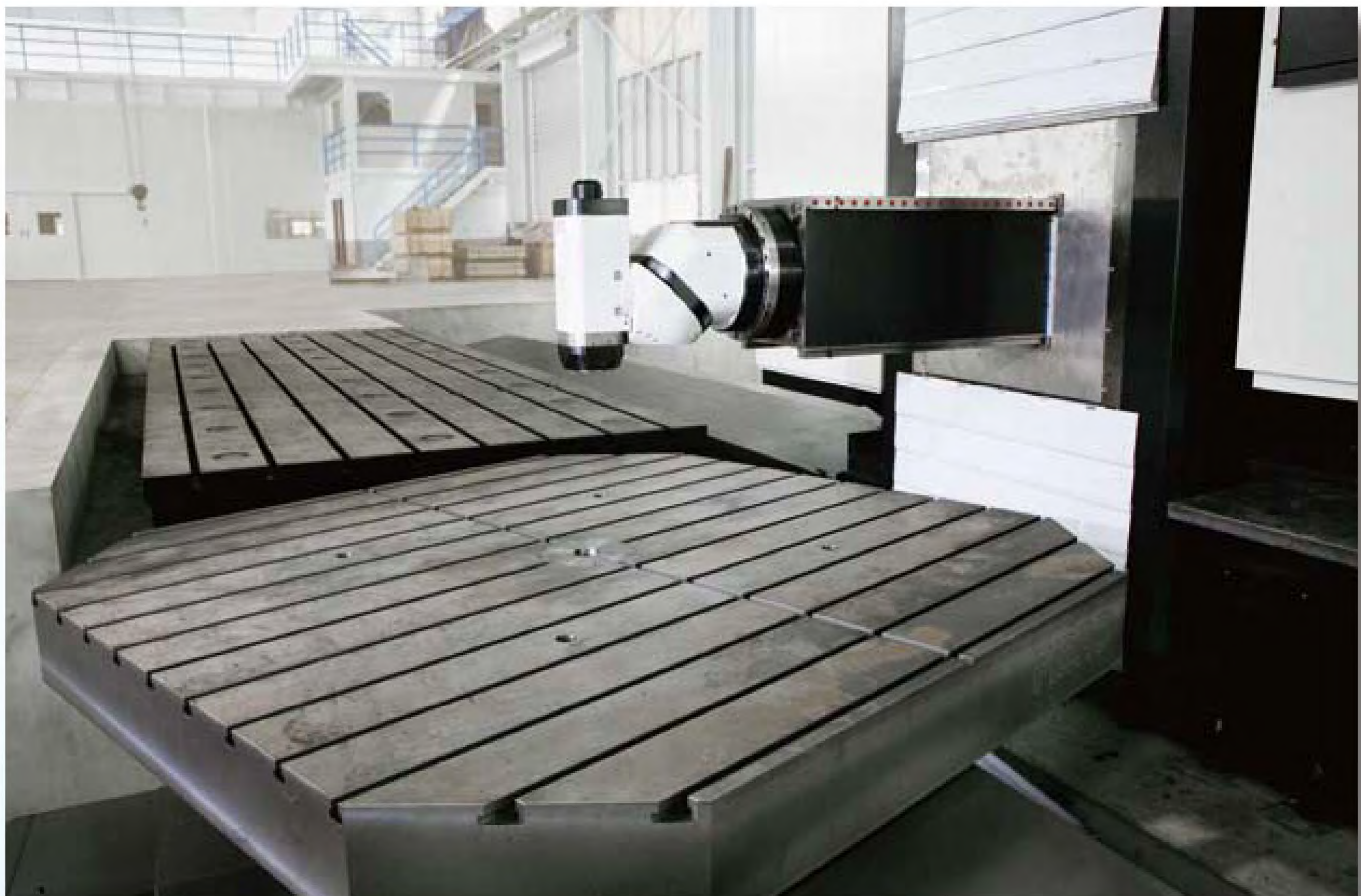
2. 7M x 2.5M x 350mm floor plate & 2.5M x 2.5M B axis CNC rotary table with 30 tons load, 5 RPM and a 1500mm V axis travel. Fully CNC 2 axes universal milling head with 34 & 42KW HSK-A100 12000RPM spindle.
