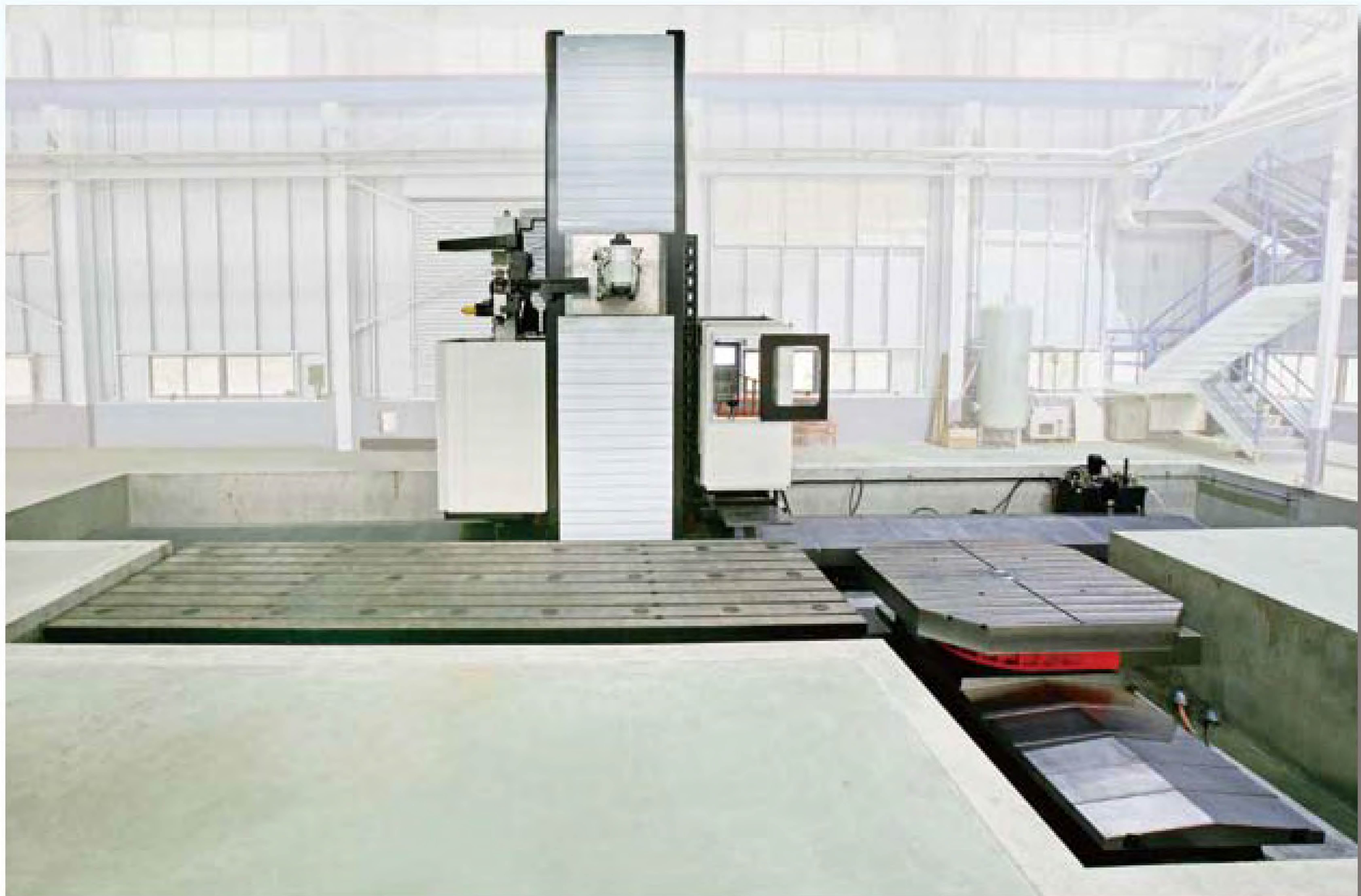
1. 10M ( X ) x 4M ( Y ) x 1.3M ( Z ) travel, 60 ATC, automatic lifting operating cabinet
