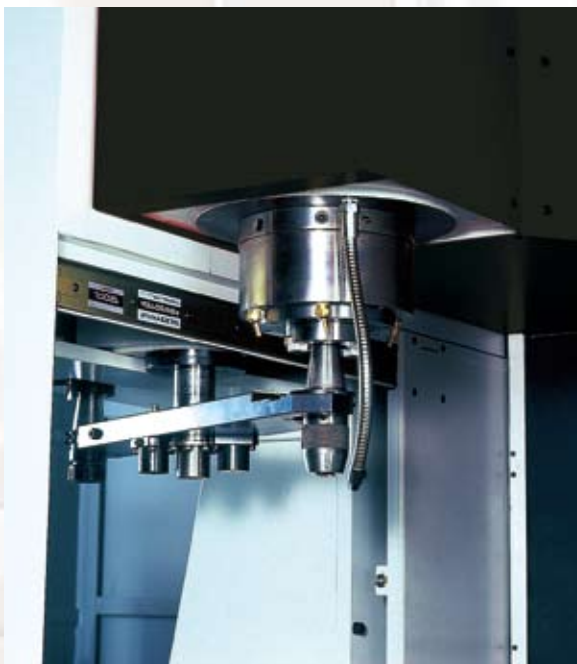
Standard Y axis 700mm travel column side mounted ATC 24 / 32 / 40 / 50 stations
