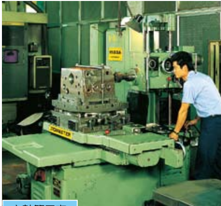
2nd finished machining for Headstock
