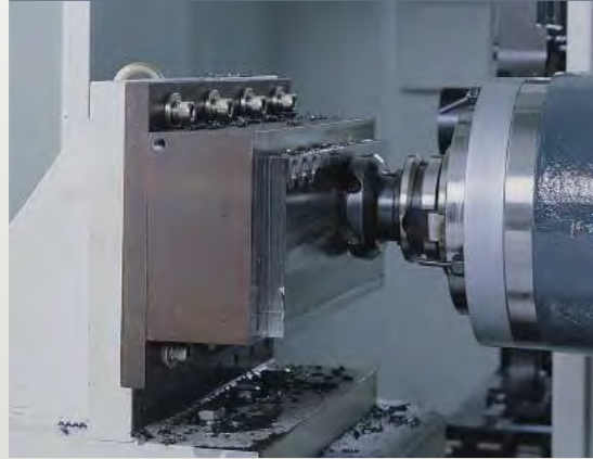
Face mill tool Ø 80mm
