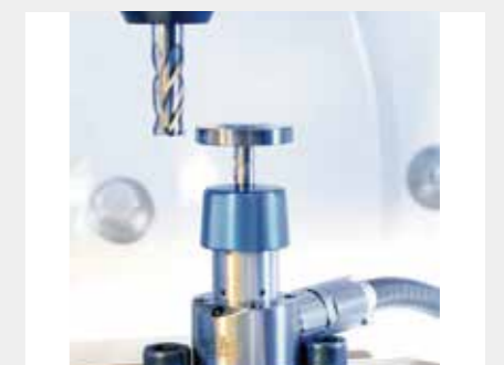
Auto. Tool Length & Diameter Measurement (m&h TS35.10) (RENISHAW RTS-27) (Optional)
