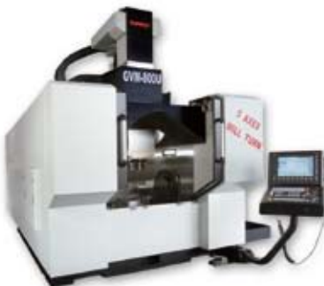
◦ GVM-800U 5 Axes gantry type machining center
