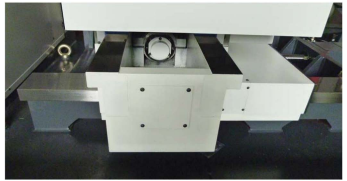
X/Z Axis Square Way Design / Z Axis Ball Screw Mounted at Central Slide
