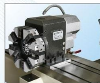
▲ Electrical system Turret
