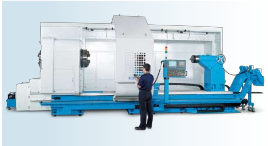
● CL-78x4000 (旋徑2500mm) Swing over bed 2500mm
