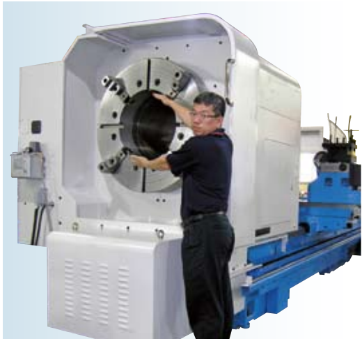
● CL-78x3000 (主軸孔徑530mm) Spindle bore 530mm
