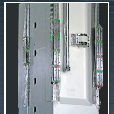
E Three linear guide ways column
