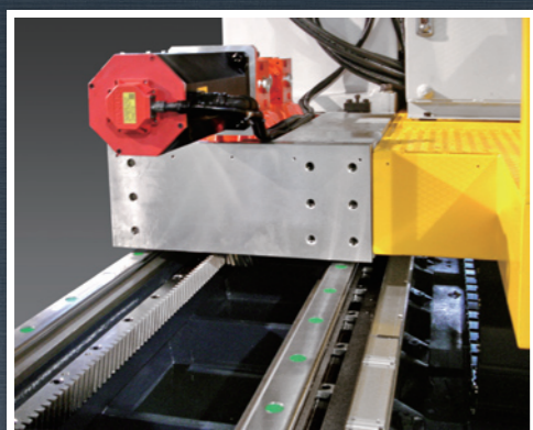
B X travel by gear-rack syn-servo control
