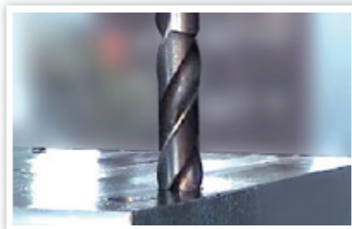
Drilling S45C Ø48mm, 1200rpm 30mm/min, Z load 80%, tolerance +0.1mm
