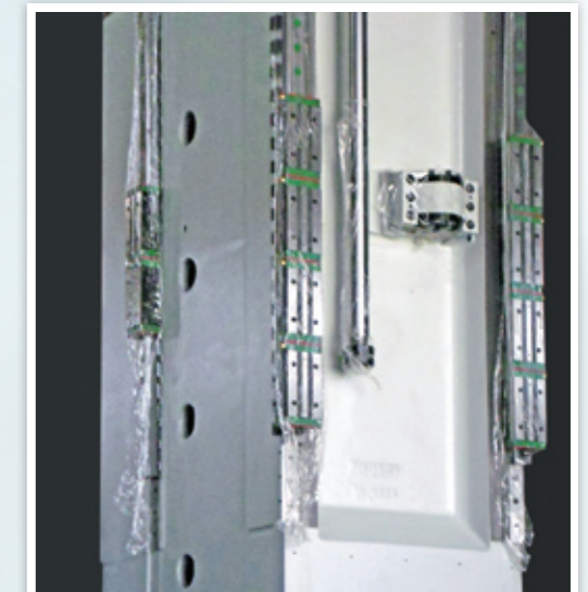
▲ Three linear guideways column
