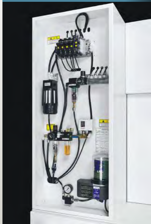
Pneumatic and Lubricant system
