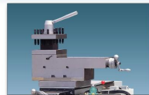
▶ 四方刀架為插掛式，可防止四方刀架反 向切削時滑動以確保安全，正反向轉動 方便 Pin-Locking Type 4-way Tool post, easy in forward and Reverse swiveling, also ensure the safety in cutting.
