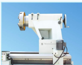
◆ Tailstock Rotary Quill Motor for Tailstock Movement 尾座迴轉心軸 尾座移動馬達
