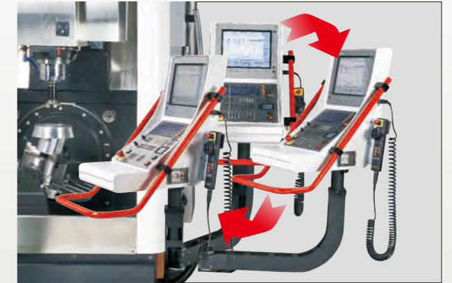
● Movable control cabinet
